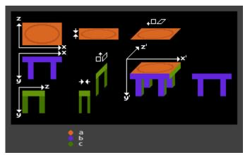
a) top view(h/2, shear along x)b) front view(taken as is)c) side view (w/2, shear along y)
